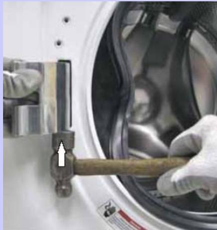
6. Push the tub assembly back while pressing the hinge arm inward and carefully remove the door hinge through the opening.
