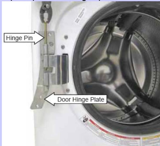
3. Remove the 3 Phillips-head screws that hold the door hinge to the front panel.
