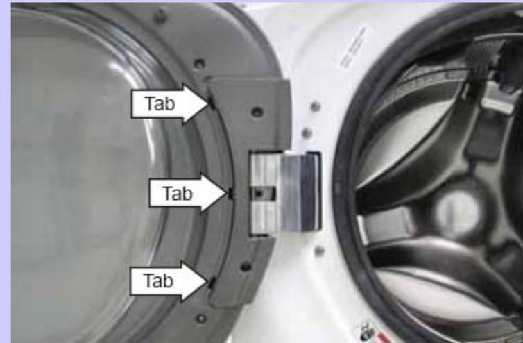
3. Remove the 2 Phillips-head screws that hold the door to the hinge door plate.
