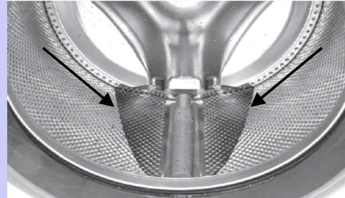
The main water level, measured behind the baffle, is approximately 2 3/4 -inches deep, and approximately 2- inches deep measured at the bottom center of the wash basket.
