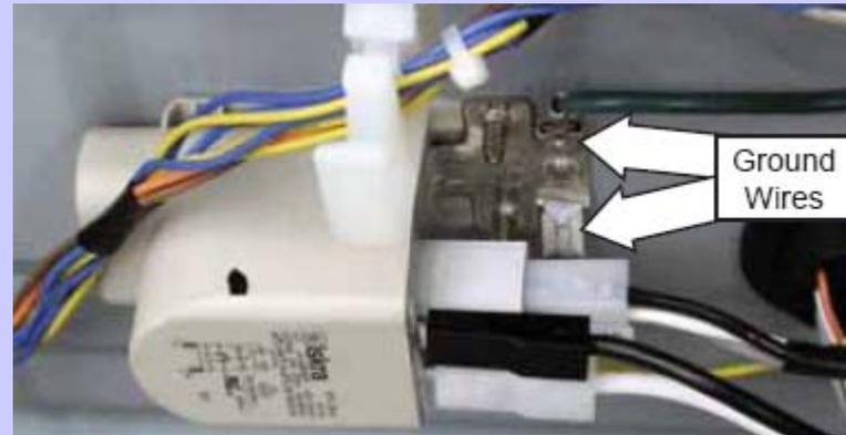
4. Remove the 2 (7-mm) hex-head screws that hold the filter to the frame.
