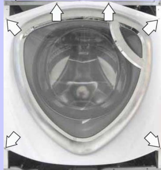
7. Lift up then remove the front panel from the 2 hooks.
