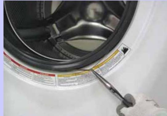
3. Remove the spring and wire from the gasket.
