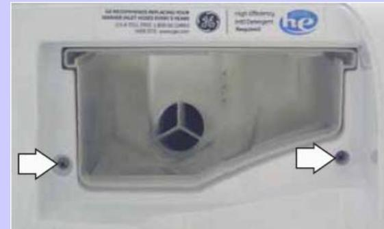
4. Remove the 3 (7-mm) hex-head screws that attach the top of the control panel to the control panel brace.
