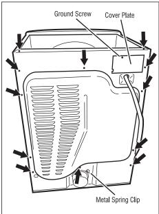
Figure 20. Remove 12 screws.
