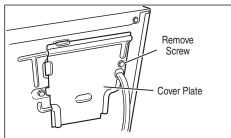
Figure 3. Remove the cover plate.
