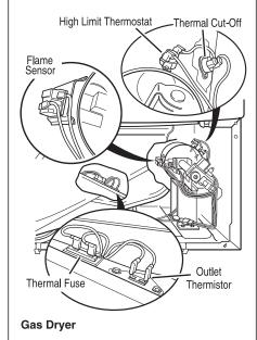
**Figure 11.** Thermal Components, viewed from front.
