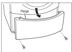
**Figure 14.** Pull the toe panel down to clear flange, then pull panel out.
