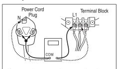
**Figure 4.** Plug-to-terminal connections for electric dryer.
