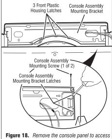
the console electronics and housing assembly.
